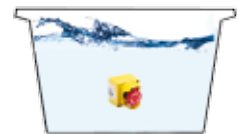
IP67: Submersion to one meter for 30 minutes.
